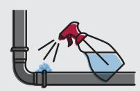
Check by doing the soap and water test. If you see bubbles forming there is a gas leak.
